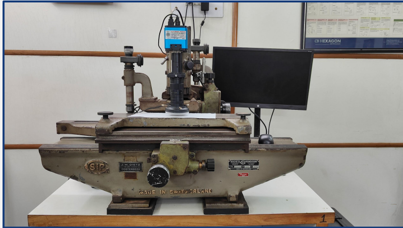
Universal Length Measuring Machine (Make: SIP Germany)
