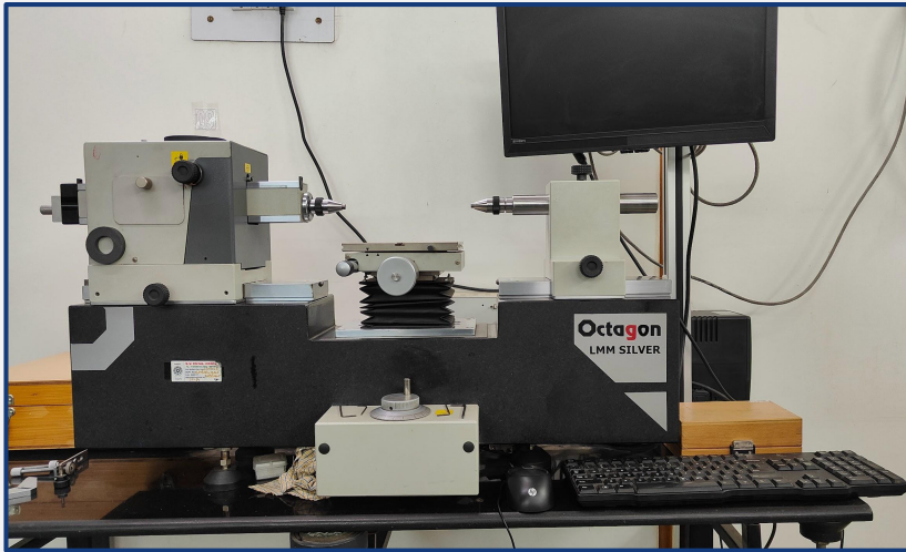
Length Measuring Machine (LMM, Make: Octagon)
