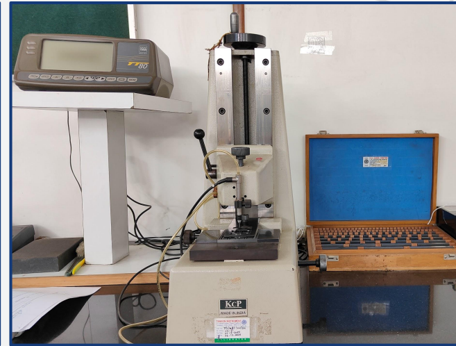
Gauge Block Comparator (Make: KPC)
