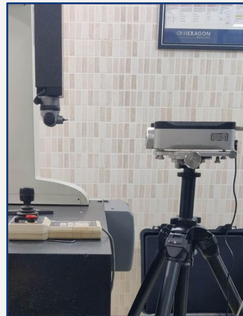
Calibration of CMM using Laser Interferometer
