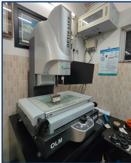
Vision Measuring Machine (Make: Hexagon)
