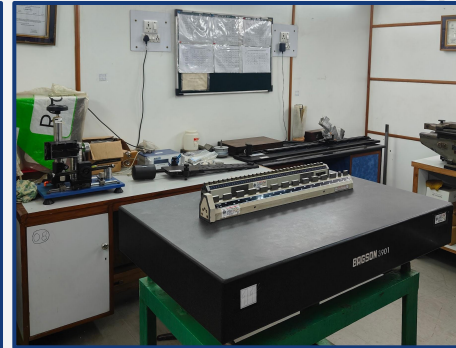
Step Gauge / Check Master with Surface Plate (Make: Micronix)
