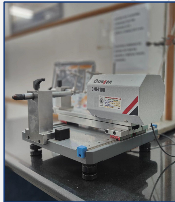
Floating Carriage Diameter Measuring Machine (Make: Octagon)
