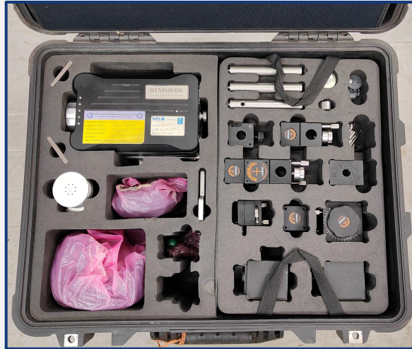
Laser Interferometer with its accessories (XL 80, Make: Renishaw)
