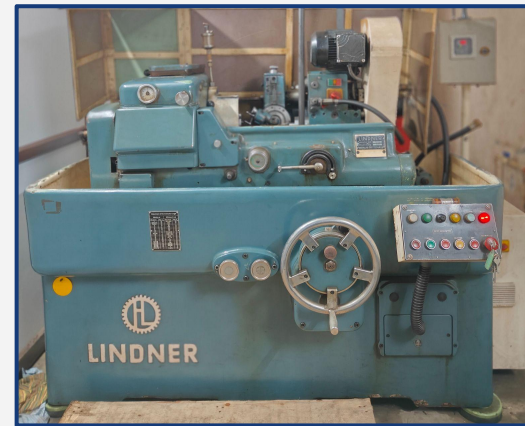
Internal Thread Grinding Machine (Make: LINDNER)
