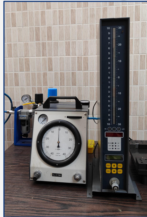
Tri Colour Column Type Air Gauge Unit
