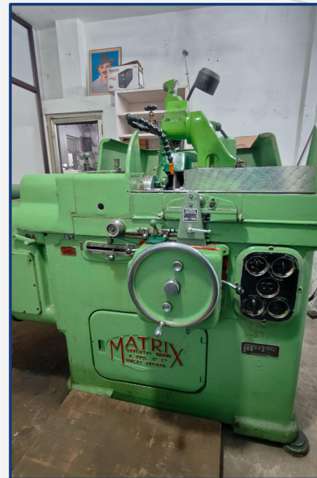
Universal Thread Grinding Machine (Make: Matrix Model: 16U)
