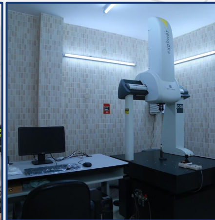
Coordinate Measuring Machine (CMM, Make: Hexagon: Brown and Sharpe, Explorer model)
