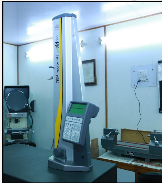
2D Height Master (Make: Tesa, Range: 600 mm)
