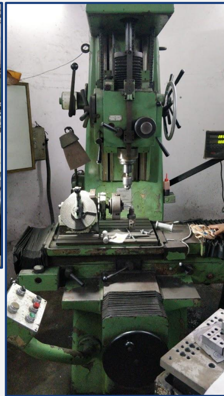
Jig Boring Machine (Make: Newall Germany)
